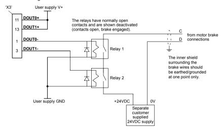
Figure 10 - Motor brake control circuit
